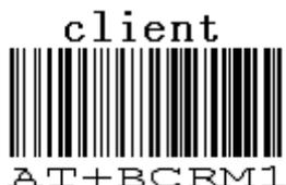
*Reading the label above can configure your Ethernet box as Client*
